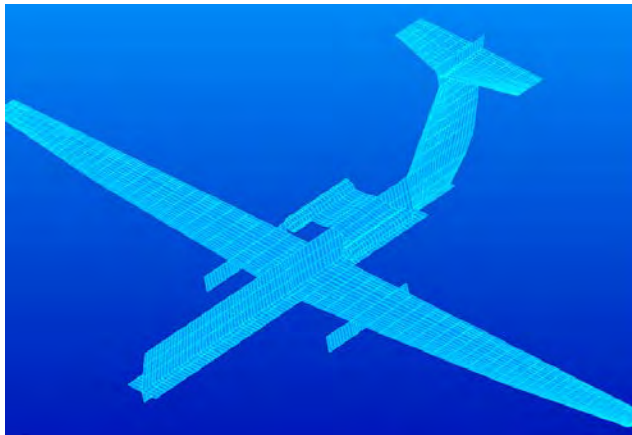
Doublet Lattice Panel Model for dynamic analysis (gust, flutter)
